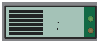
Level Gauge ON Digital Timer Readout OFF LEDs OFF
