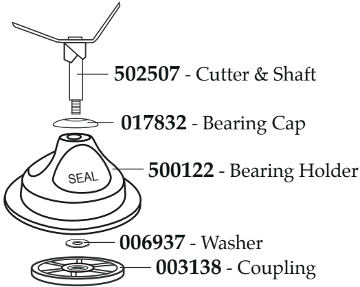
Parts for the 502508 Blending Assembly (that can be purchased separately)
