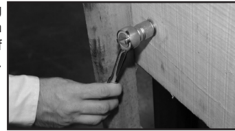
Removing skid from bottom of cabinet.
