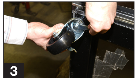
Use the tool provided to tighten the castor into place.
