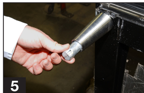
The end of the leg is adjustable to easy leveling.
