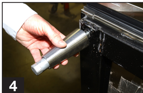
Thread leg into cabinet bottom frame rail.
