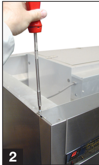
2 Three Door Freezer unit (Rainshield Removal/top screws)
