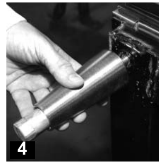
4 Thread leg into cabinet bottom frame rail.
