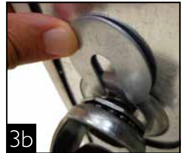
Installing castors (shims)
