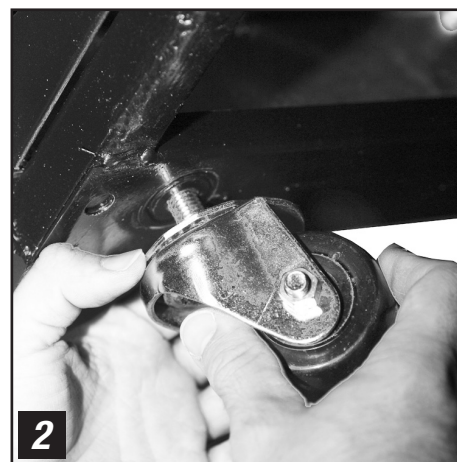
2 Thread castors into existing leg leveler holes.
