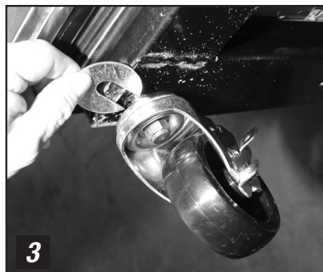
3 Use shims as necessary to level cabinet.
