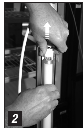
2 Remove bulb by gently pulling up on spring loaded lampholder.
