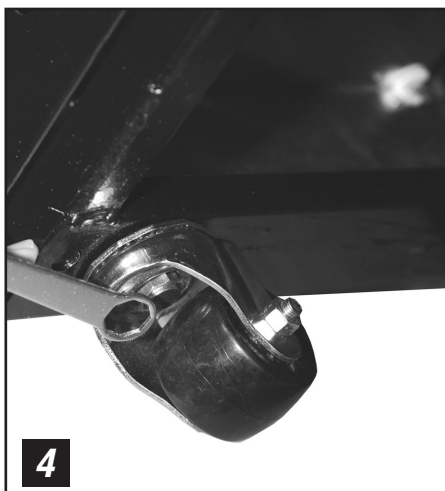
4 Tighten castor in position with castor wrench.
