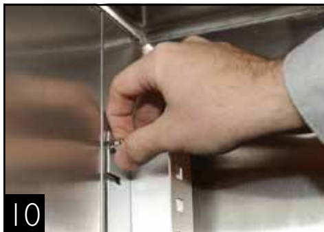
Pilaster installation (side wall of cabinet)
