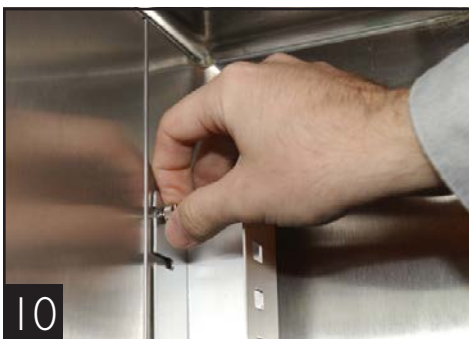
Pilaster installation (side wall of cabinet)
