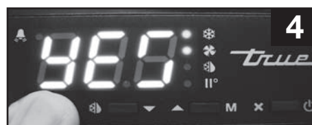
Image 4: If "yes" appears on screen, the controller is locked.
