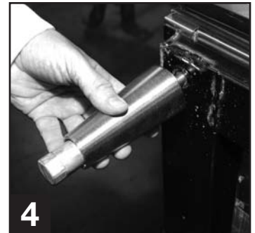
4 Thread leg into cabinet bottom frame rail.
