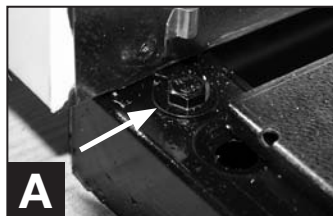
Removing skid from bottom of cabinet.
