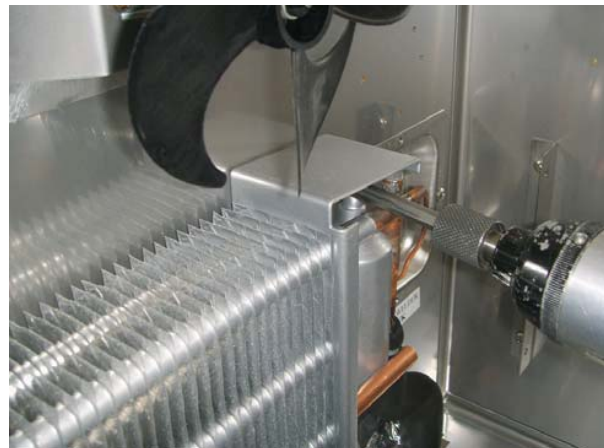
A. Remove the evaporator coil
