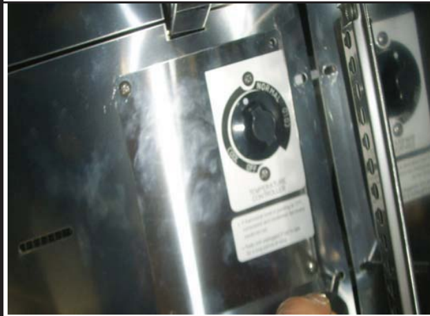
C. Remove the temperature & sensor
