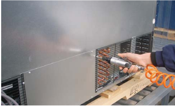
B. Disassembly the condensing unit
