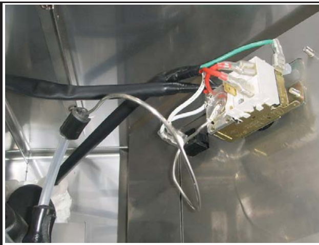
C. Remove the temperature & sensor
