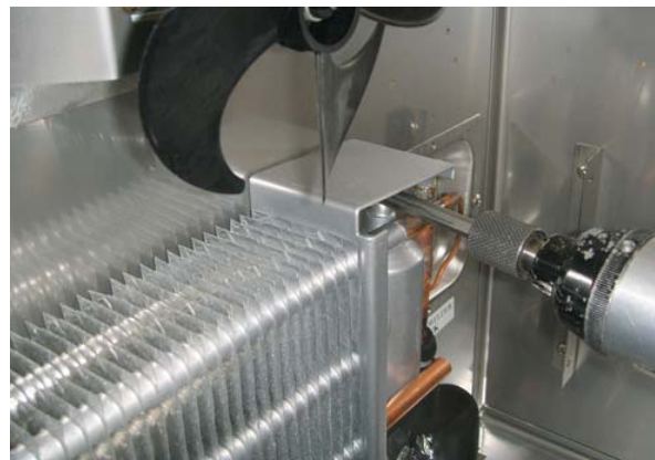
A. Remove the evaporator coil
