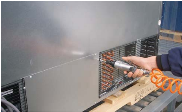
B. Disassembly the condensing unit
