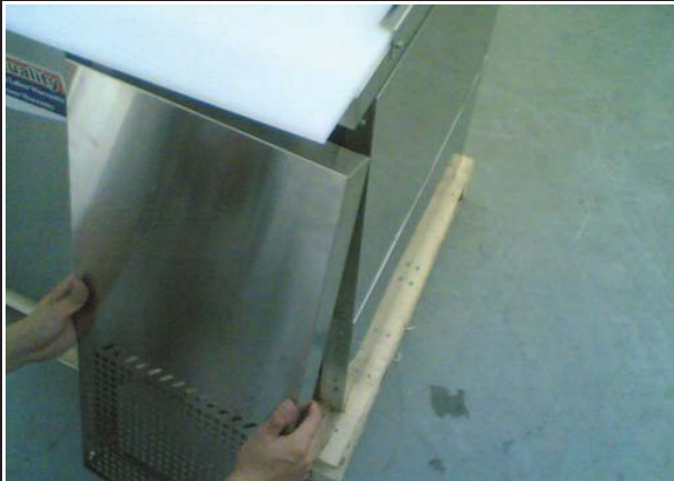
C.Remove the unit front cover
