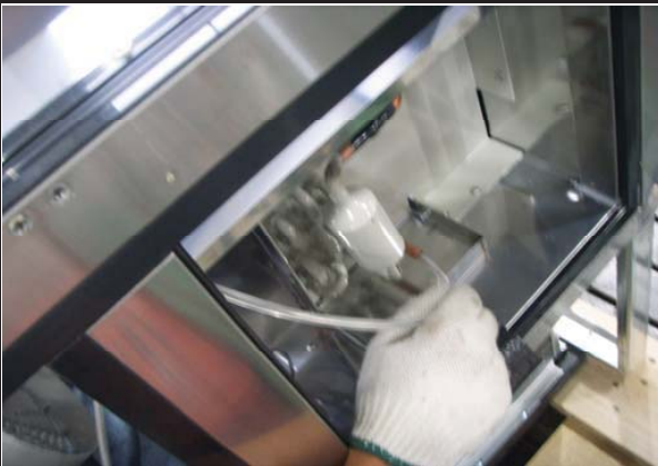
E.Remove the evaporator coil
