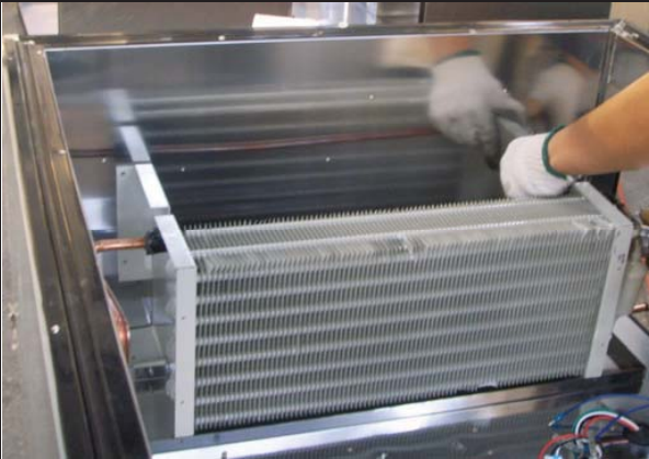
E.Remove the evaporator coil
