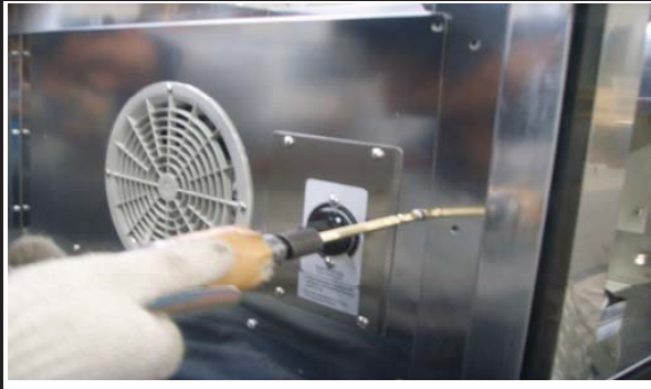
B.Disassemble the evaporator front duct panel
