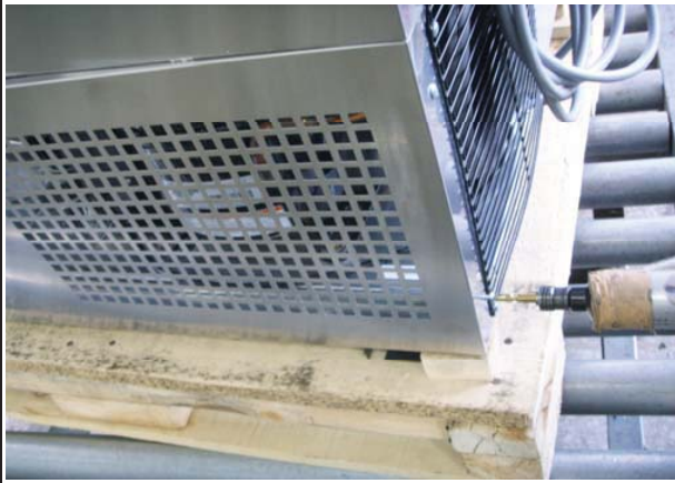
C.Remove the unit front cover
