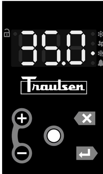
Fig. 6B.14.2b DISPLAY DURING ELECTRIC DEFROST
