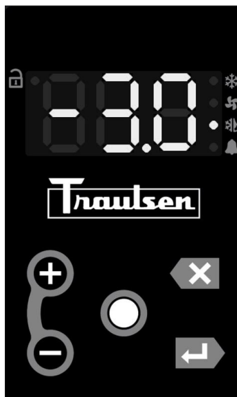
Fig. 6B.14.2c DISPLAY DURING FREEZER ELECTRIC DEFROST
