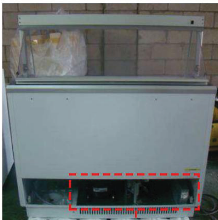
Photo 10 - Machinery compartment view of model TIDC-47W
