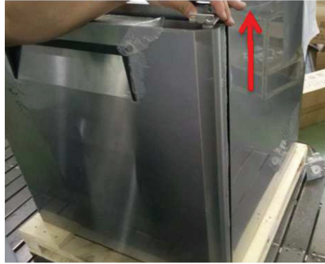
2) Remove the top hinge from the unit.
