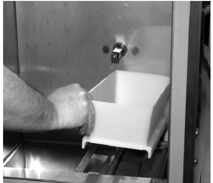
Figure-11 Accumulator Housing
