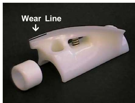
Figure 12. Auger Flight Wear & Front Auger Support Bushing Wear
