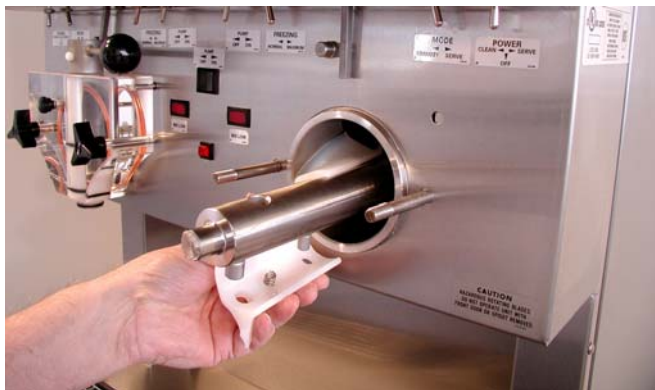
Figure 14. Auger Flight Removal
