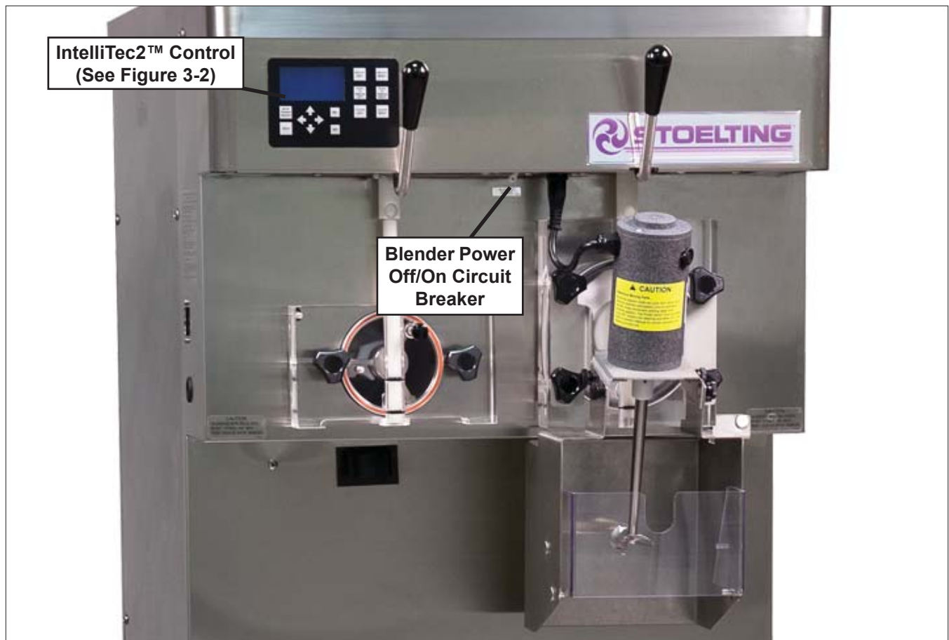
Figure 3-1 SU444 Freezer Controls
