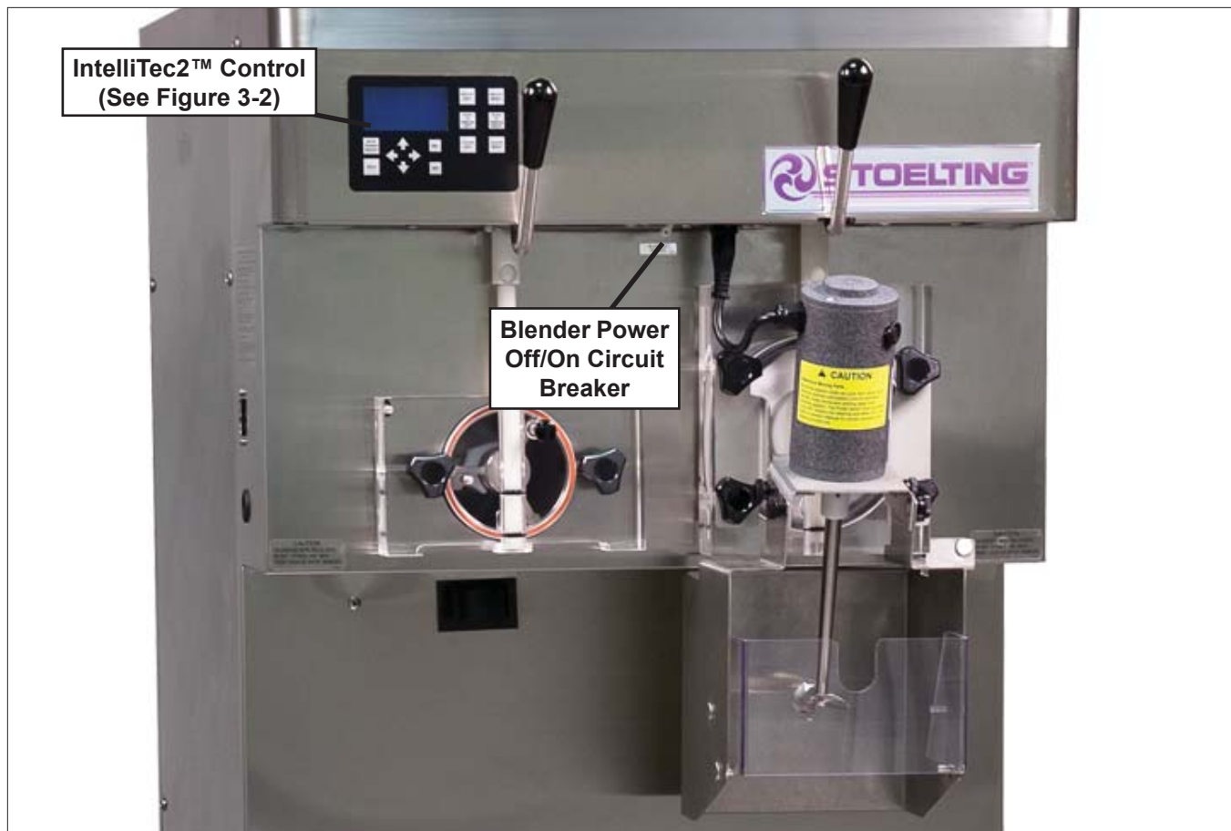
Figure 3-1 SU444 Freezer Controls
