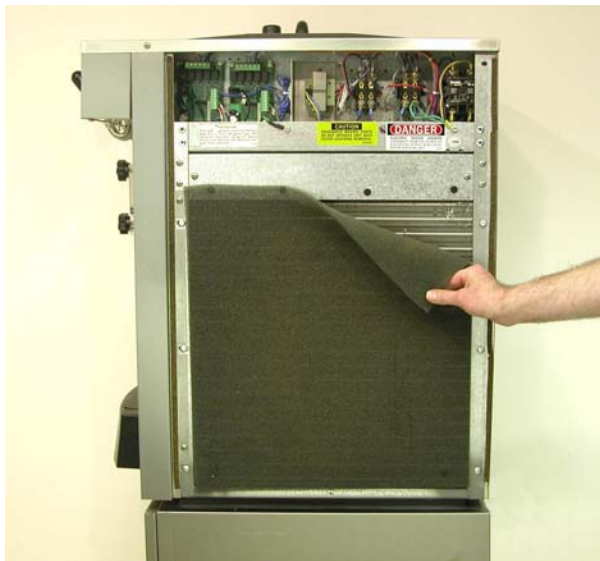
Figure 4-5 Condenser Filter Removal
