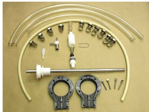
Figure 3-10 Mix Pump Removable Parts
