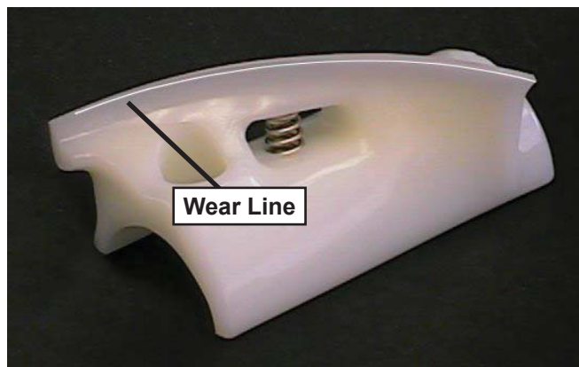
Figure 3-3 Auger Flight Wear
