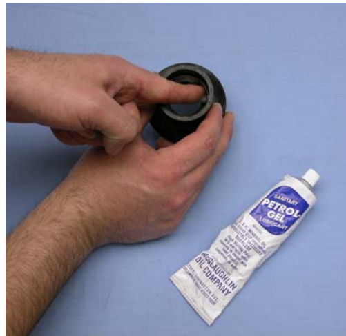
Figure 3-6 Lubricate Rear Seal
