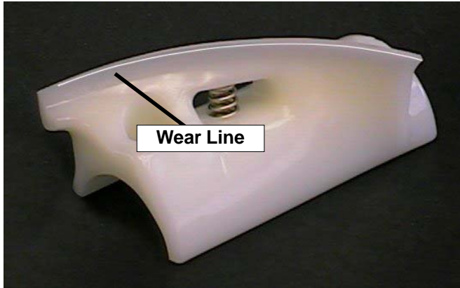
Figure 3-3 Auger Flight Wear
