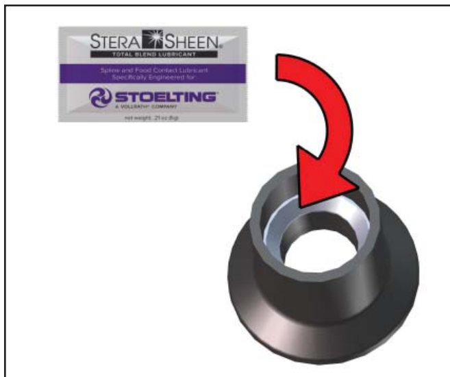
Figure 3-6 Lubricate Rear Seal
