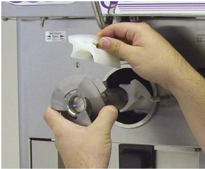
Figure 3-8 Removing Auger Shaft and Flights
