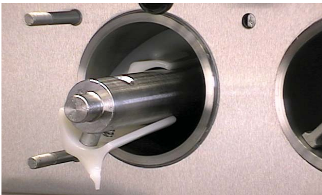
Figure 3-5 Auger Flight Removal
