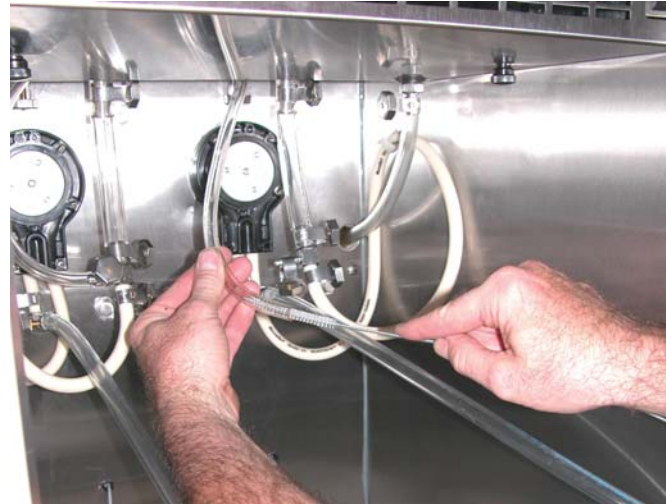
Figure 3-18 Cleaning Air Tube
