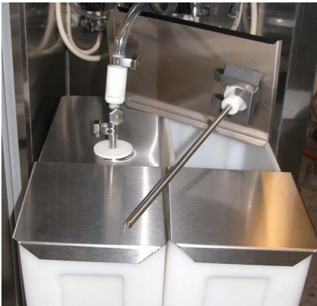
Figure 2-5 Connecting Mix Pick-up Assembly
