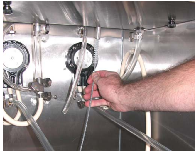
Figure 3-19 Cleaning Feed Tube
