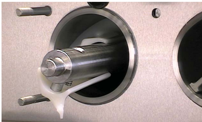
Figure 3-5 Auger Flight Removal
