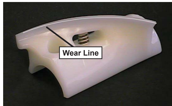
Figure 3-3 Auger Flight Wear
