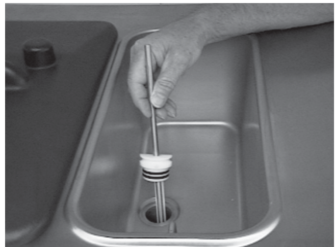
Figure 17. Removing Mix Inlet Regulator
