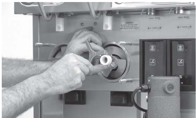
Figure 24. Removing Auger Supports
