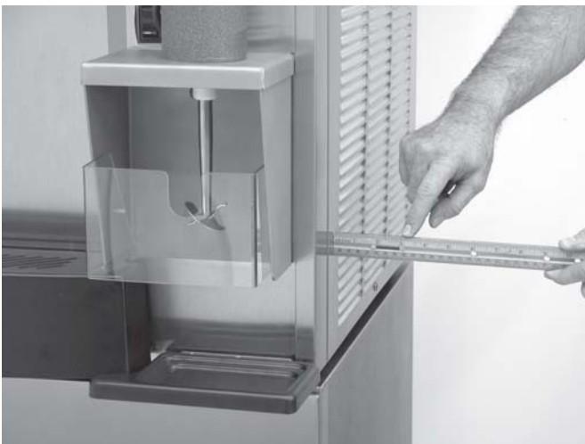
Fig. 4. Space and Ventilation Requirements
