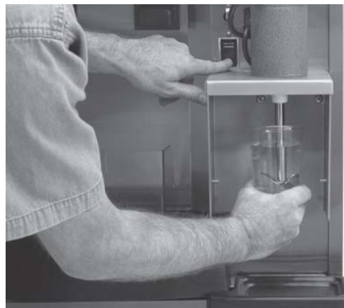
Figure 18. Cleaning Agitator Shaft
