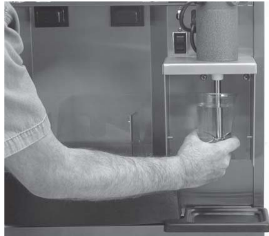
Figure 14. Sanitizing Agitator Shaft (SF144 Model Only)
