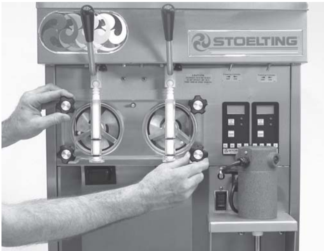
Figure 20. Removing Front Door
