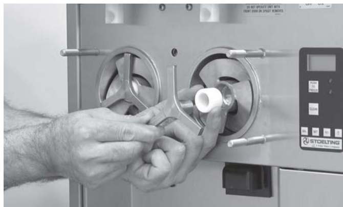
Figure 23. Removing Auger Supports
