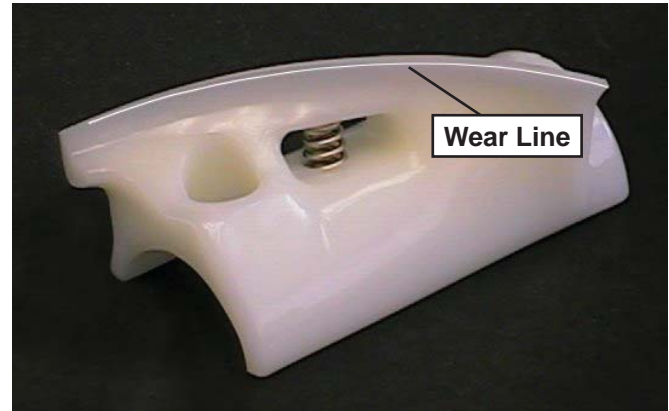
Figure 3-3 Auger Flight Wear
