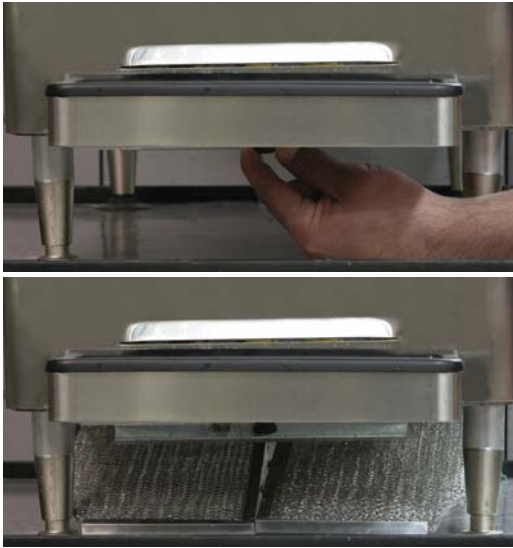
Figure 3-10 E112 Condenser Filter Removal
