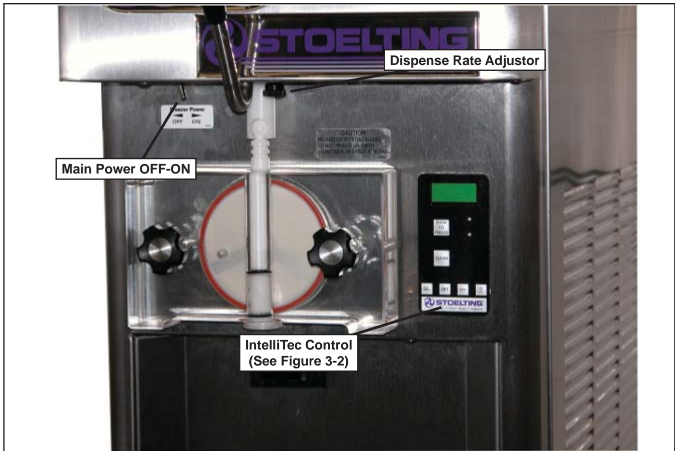
Figure 3-1 E111 & F111 Controls
