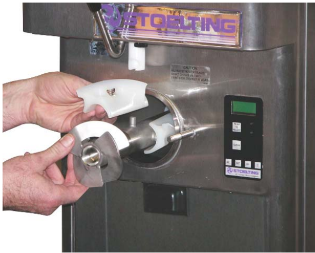
Figure 3-5 Removing Auger Shaft and Flights
