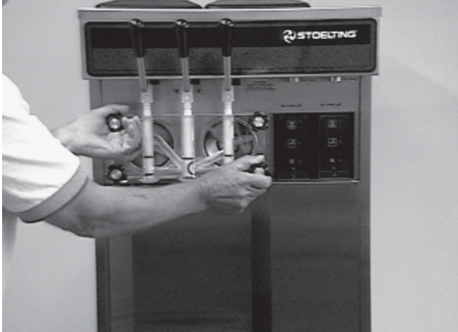
Figure 19. Removing Front Door
