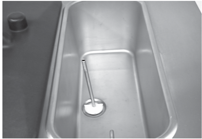
Figure 26. Install Mix Inlet Regulators
