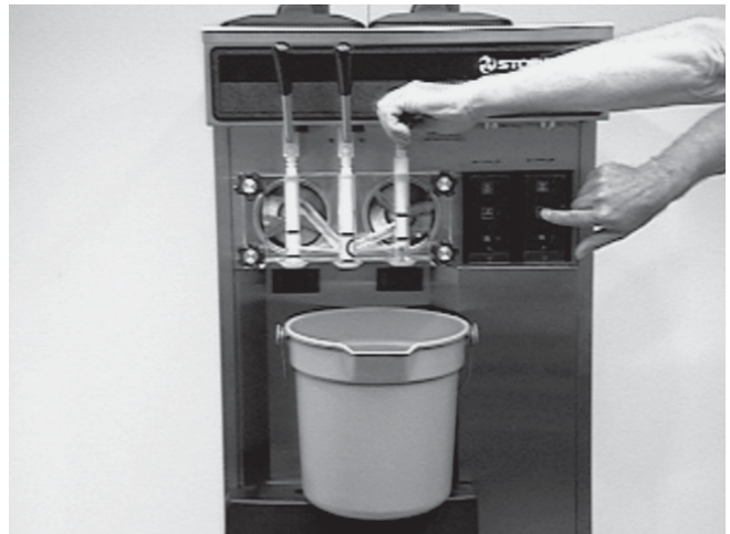
Figure 14. Spigot Opened and Solution Draining
