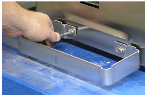
Figure 2-3 Drip Tray Bracket
