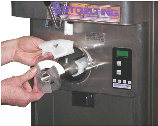
Figure 3-5 Removing Auger Shaft and Flights
