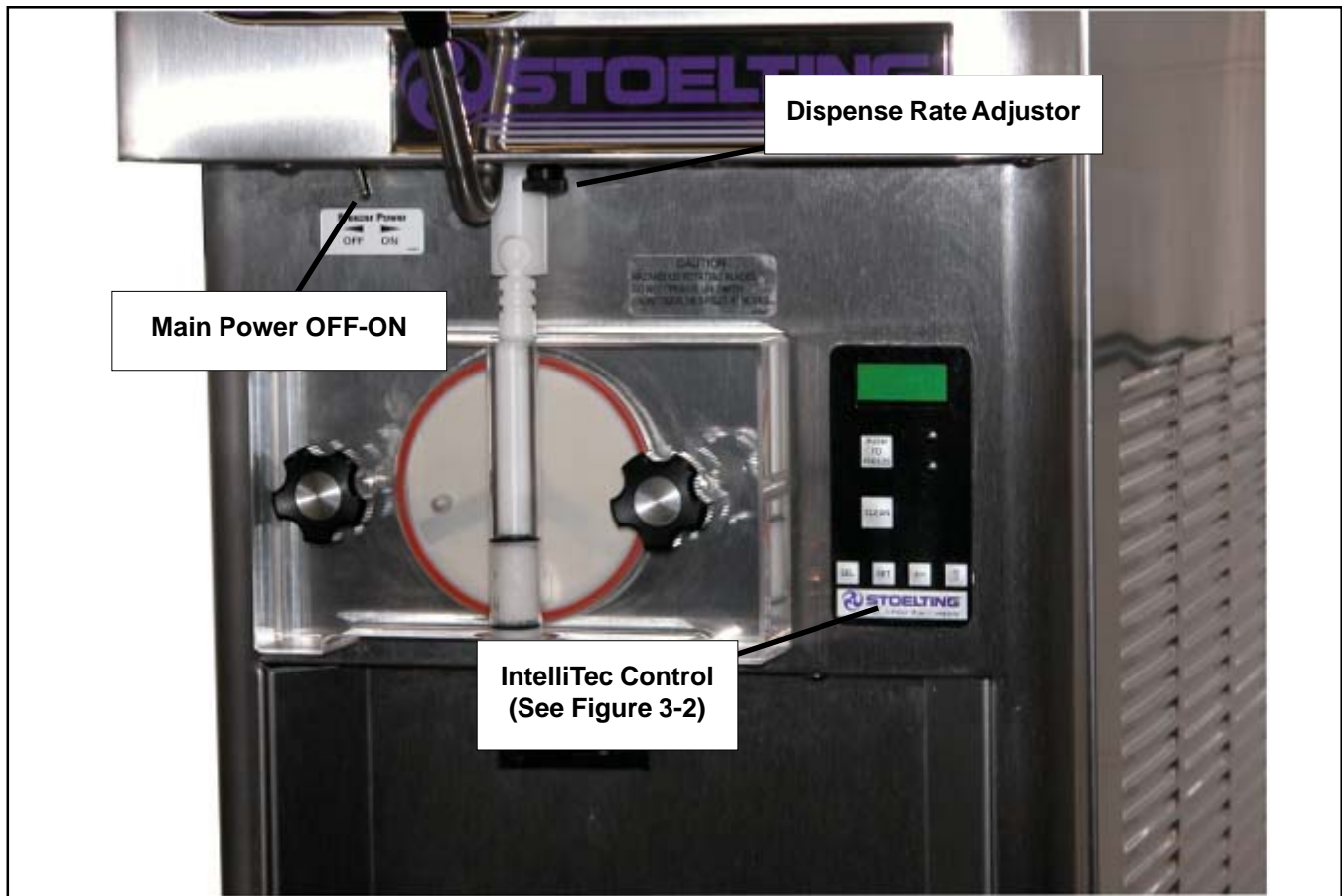
Figure 3-1 E111 & F111 Controls
