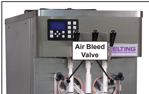
Figure 3-8 Air Bleed Valve
