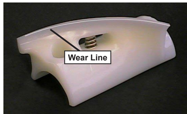
Figure 3-3 Auger Flight Wear
