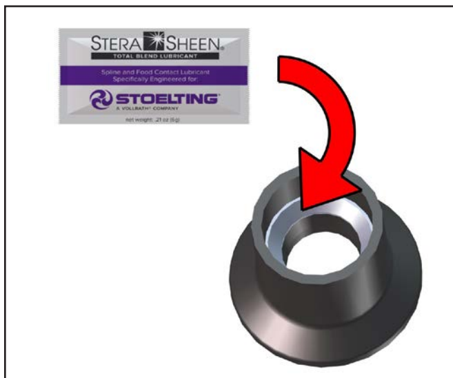
Figure 3-6 Lubricate Rear Seal
