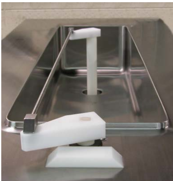
Figure 3-3 Flow Control Assembly
