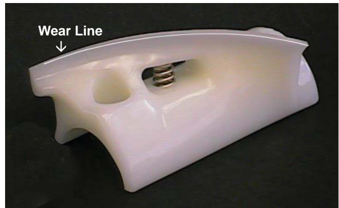
Figure 3-3 Auger Flight Wear
