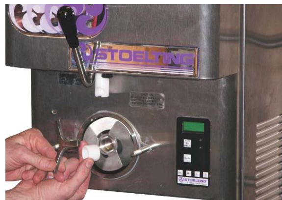
Figure 3-4 Removing Auger Support
