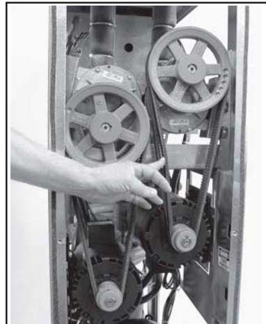
Figure 21. Belt Adjustment (Model 237 Shown)
