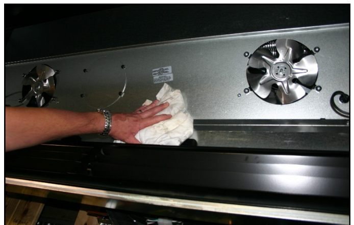
Image #2 Clean under Air Return Grille and Fan Shroud Area with moist cloth. Remove drain cleaning access door and clean drain.
