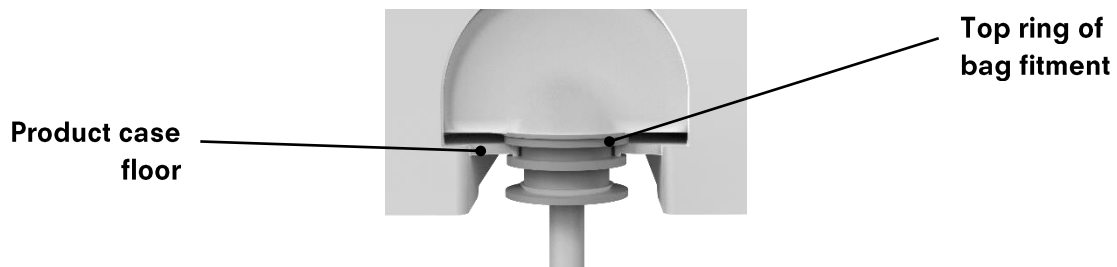
Figure 20: Top ring of bag fitment must be resting on product case floor
