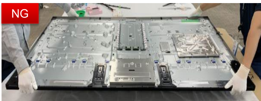
Carry P-mod by horizontal position
