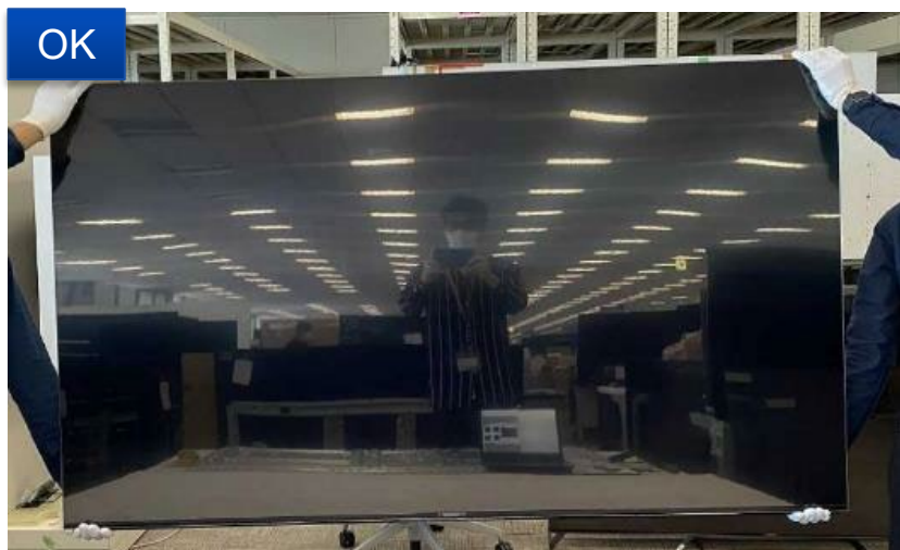
Carry P-mod by vertical position
