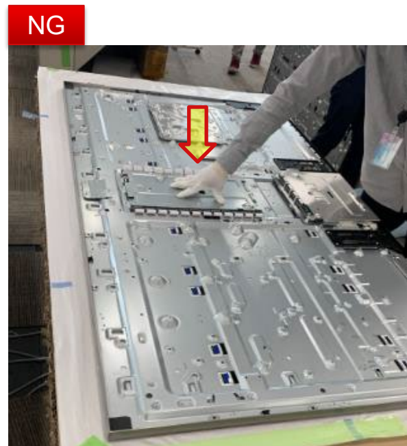
Press on P-mod during Assy & Disassy
