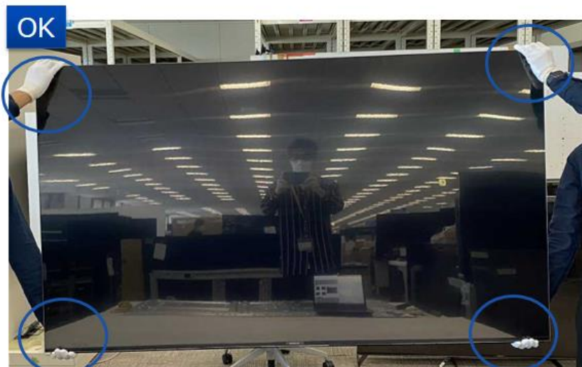
Always wear gloves during P-mod handling
