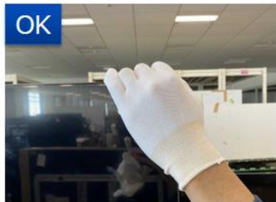
Holding edge of BZ without touching o-cell
