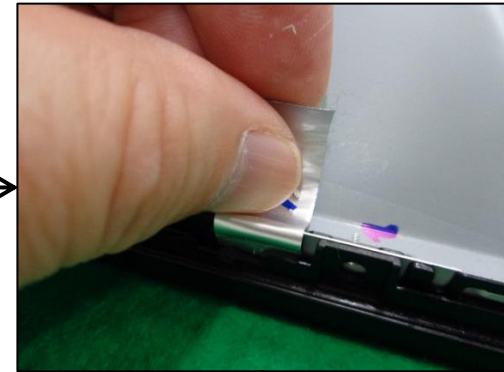
Paste Aluminum-Tape to LCD-Panel)
